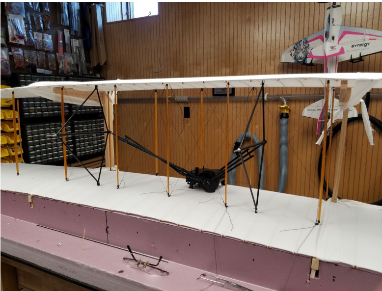
Wing— Permanent assembly with prop supports, engine, chain guides and rigging. View from the back.
