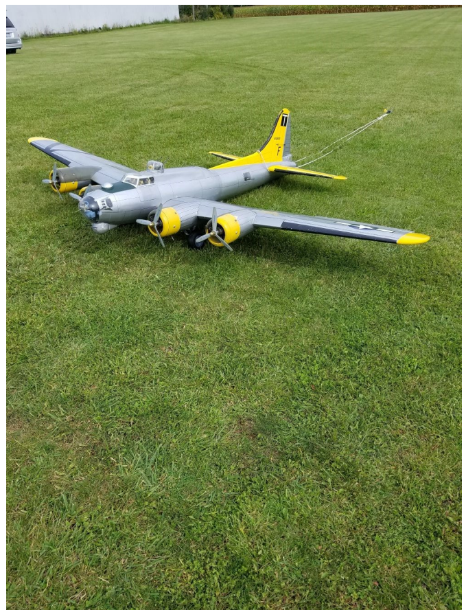
This flew at the FLAPS show. 10ft wingspan, (4) OS 91 4-strokes, 50Lbs.
