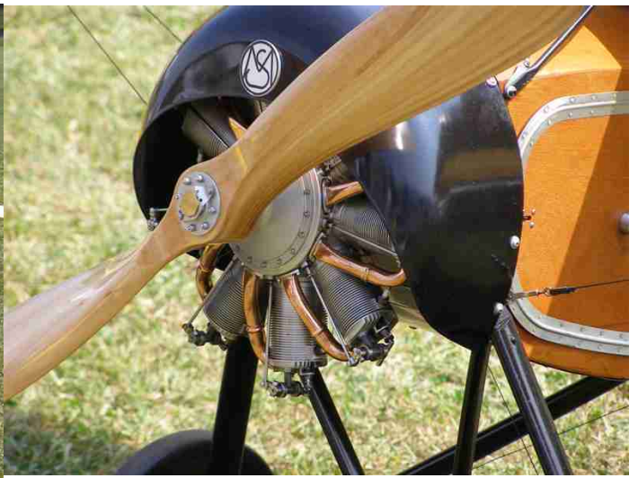
Functioning model of a LeRhone Rotary engine- Took 4 years to build The cylinders spin with the prop
