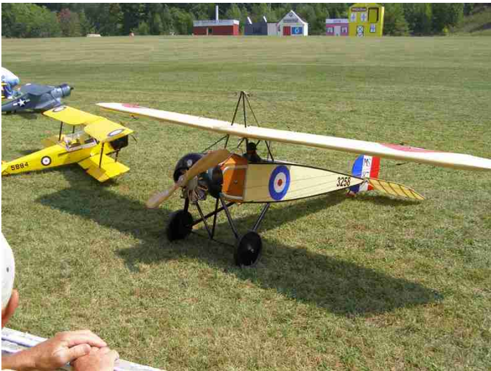
Functioning model of a LeRhone Rotary engine- Took 4 years to build The cylinders spin with the prop
